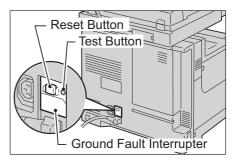
**6** Press the <RESET> button back to the depressed position.
